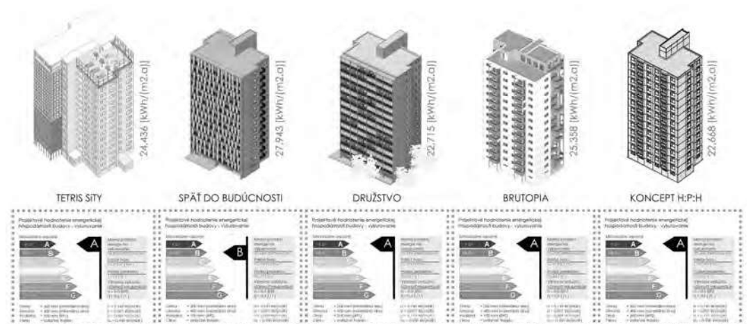
Fig. 7.: Comparison of specific heat demand calculations for heating individual designs (Zdroj: Roman Ruhig)
