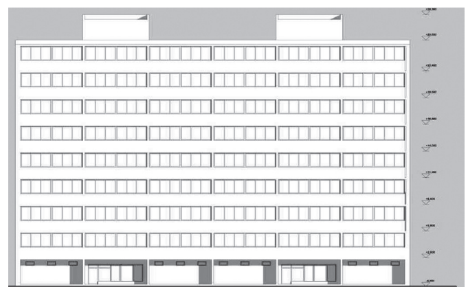
Fig. 5 Variant 4 - Front view of the T 08 B apartment building - interconnection of the loggia into the heated volume capacity (Source: Ruhig, 2020)
